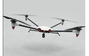
It pulls together staff and students from aerospace, robotics, and product design within UWE to deliver a drone with take-off weights right up to the current legal limit of 7kg. It is currently fitted with a tracking camera but is cable of carrying an array to tailored technologies being developed.
